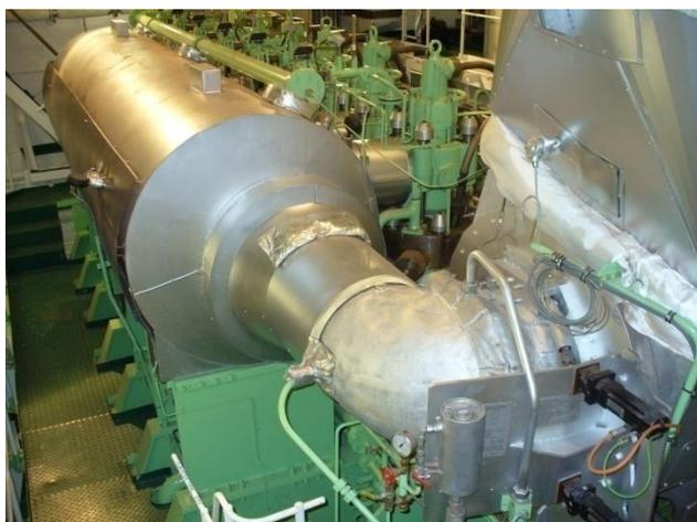
*The MAN Diesel axial TCA55-2V turbocharger with VTA technology on a six cylinder, 46 cm bore MAN B&W type 6S46MC-C two stroke engine aboard the shallow draught tanker Stena President. The VTA turbocharger recently achieved 10,000 operating hours. A thorough inspection revealed excellent findings*
