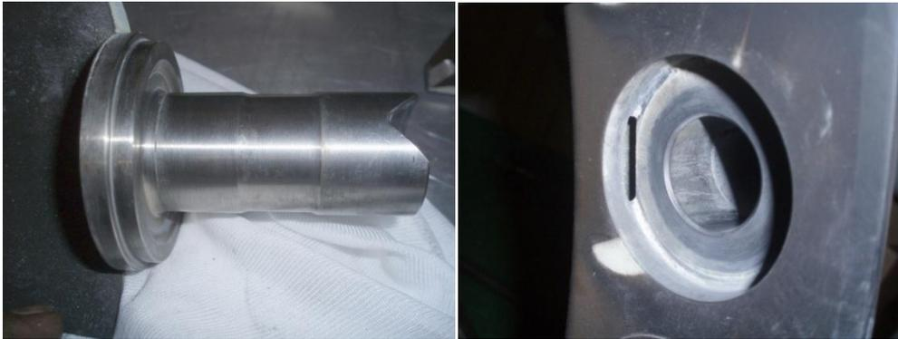
*(left and right) After 10,000 operating hours in the TCA55-2V turbocharger with VTA technology, the bearing surfaces of both the adjustable nozzle ring vanes (left) and their seats (right) were still within their original works dimensional tolerances*
