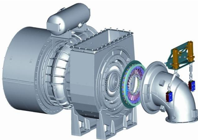
*VTA turbochargers from MAN Diesel feature a nozzle ring with adjustable vanes. Seen here is the axial variant for the TCA axial turbocharger. The system is modular and occupies the same position as a fixed nozzle ring. It can be retrofitted to turbochargers already in the field*
