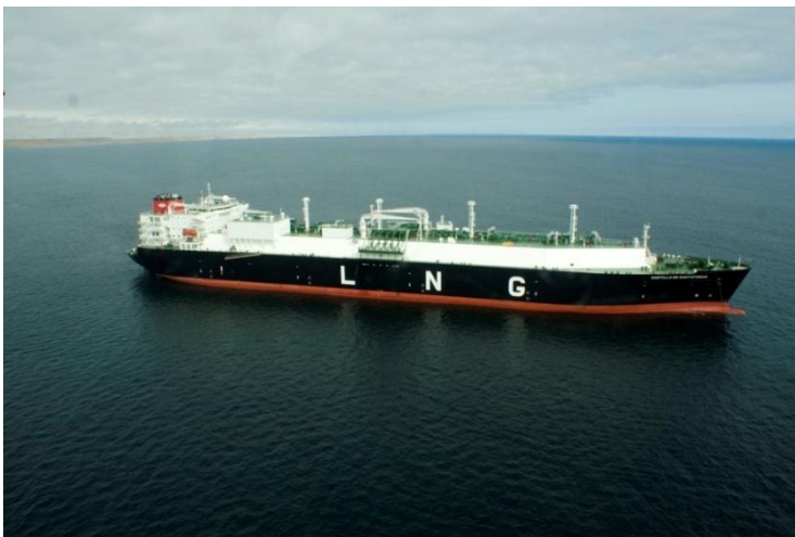
The LNG carrier Castillo de Santisteban is powered by five dual-fuel MAN 8L51/60DF engines
