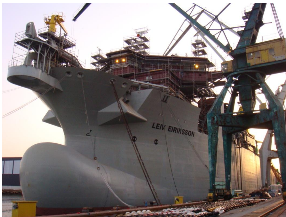
The Leiv Eiriksson pictured during construction at La Naval shipyard in Sestao, Spain. An Alphasonic 2000 propulsion management system controls the dredger's entire propulsion package that includes two MAN Diesel Alpha-type VBS1680-ODF propellers operating in nozzles. The propellers' blade feet and hub are partly chromium-coated for protection against abrasive wear and calculated bollard pull is an impressive 560 metric tons
