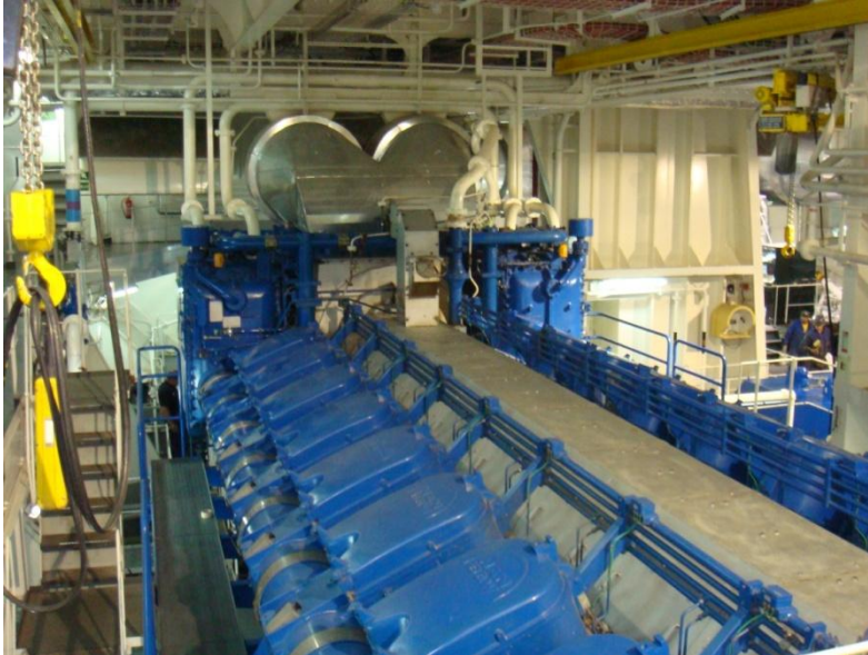
View of the 16V48/60B main engine within Cristóbal Colon's engine room
