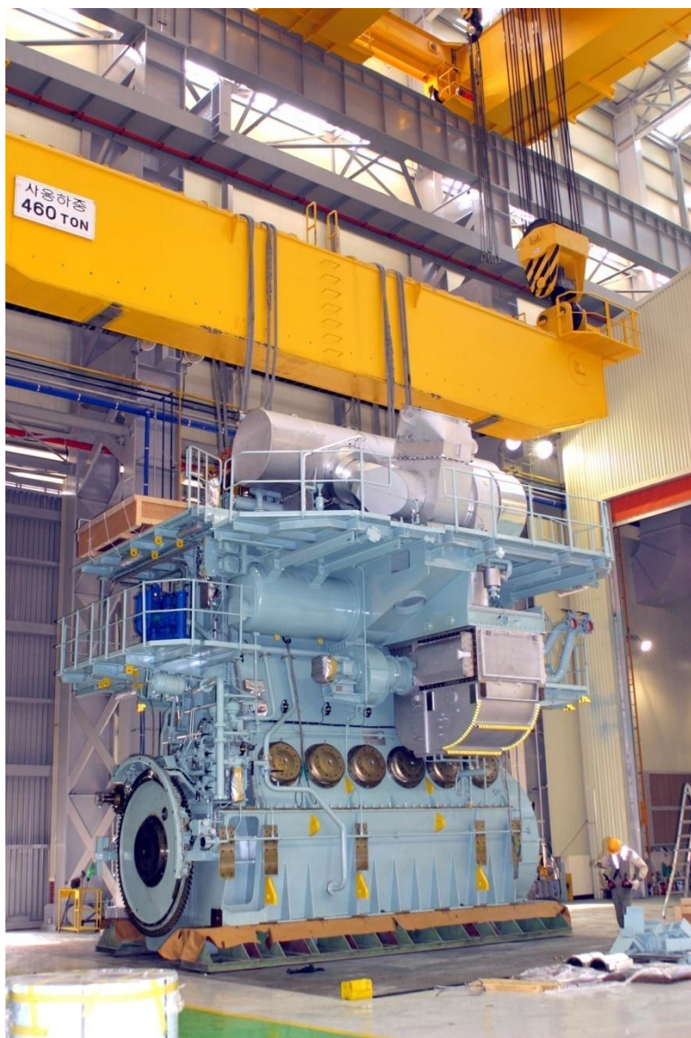
A 6S50ME-C engine pictured after production at STX
