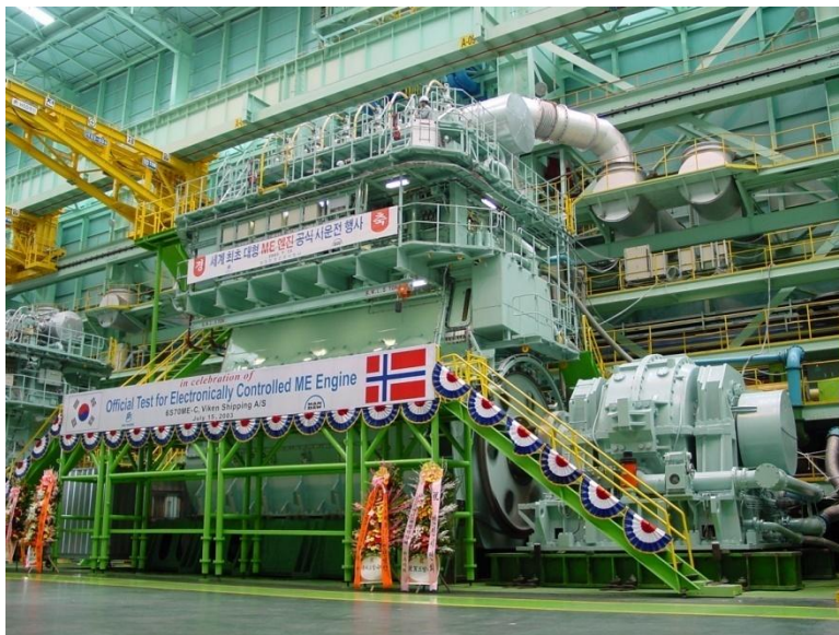
A 6S70ME-C engine pictured on the testbed at Doosan
