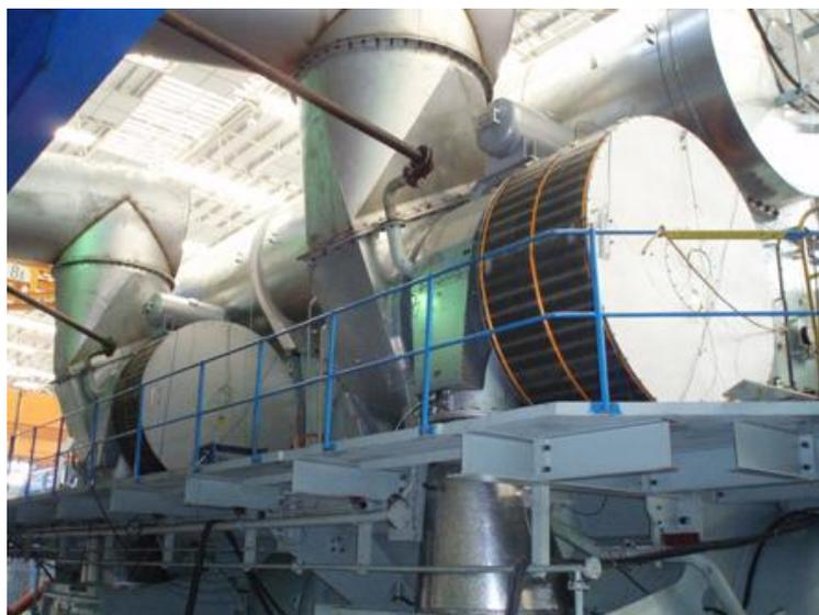
*Two MAN Diesel TCA88-25 axial turbochargers mounted on a low speed two stroke of MAN B&W brand 8K98MC engine built under licence by CMD in Shanghai. The engine will power a 5,100 TEU container vessels presently under construction at Jiangnan Shipyard in China for COSCO.*
