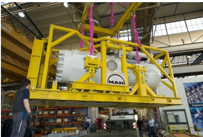
Subsea HOFIM™ Kompressor von MAN Diesel & Turbo – © MAN Diesel & Turbo
