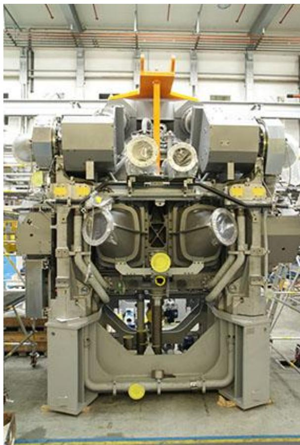
*Frontal view of ECOCHARGE two-stage turbocharging system featuring 2 x TCR20 and 2 x TCX17 turbochargers*
